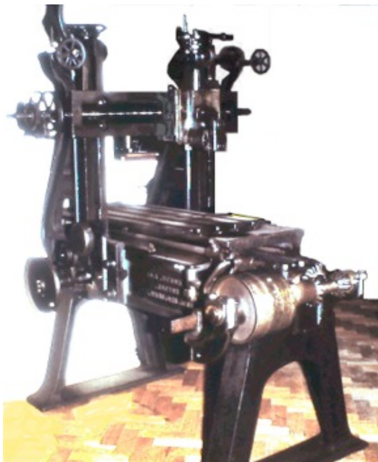
The 1842 Whitworth Planing Machine.
