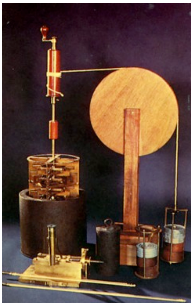
Replica of Joule's paddlewheel experiment.
