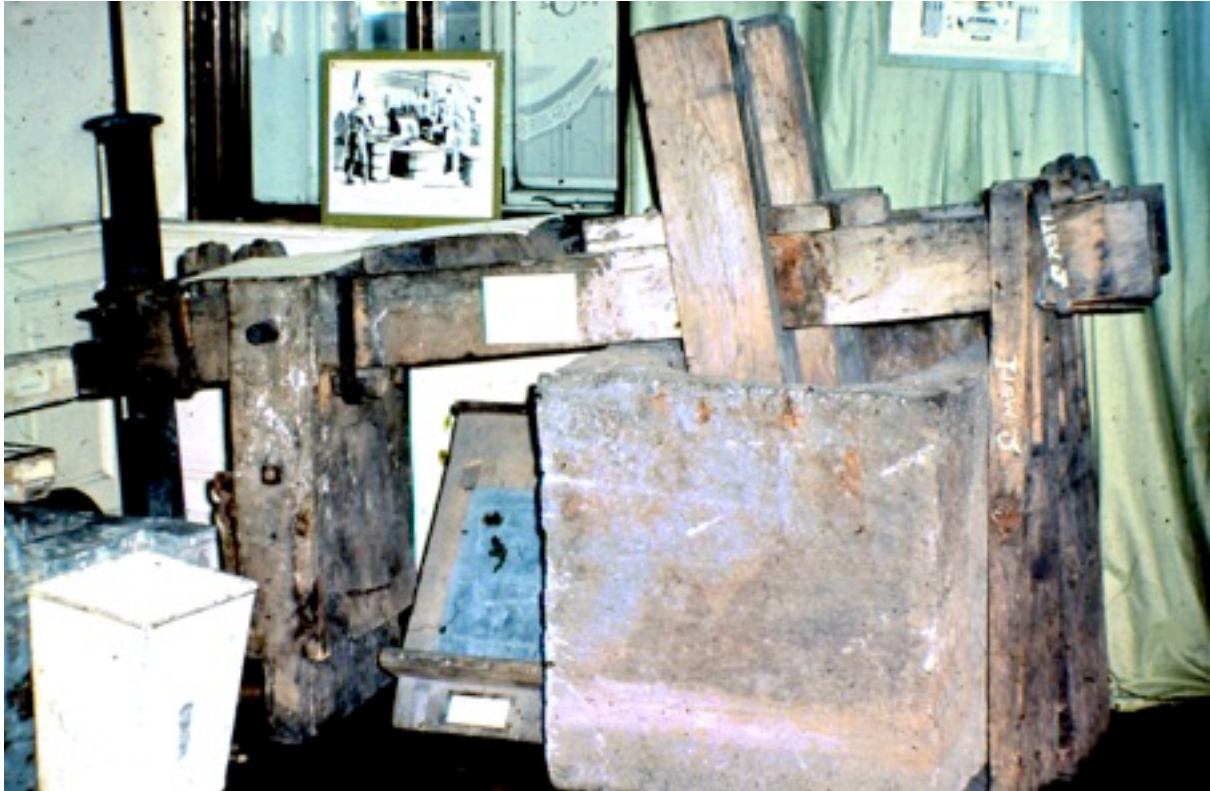
The stampers with their stone trough on display at Grosvenor Street.
