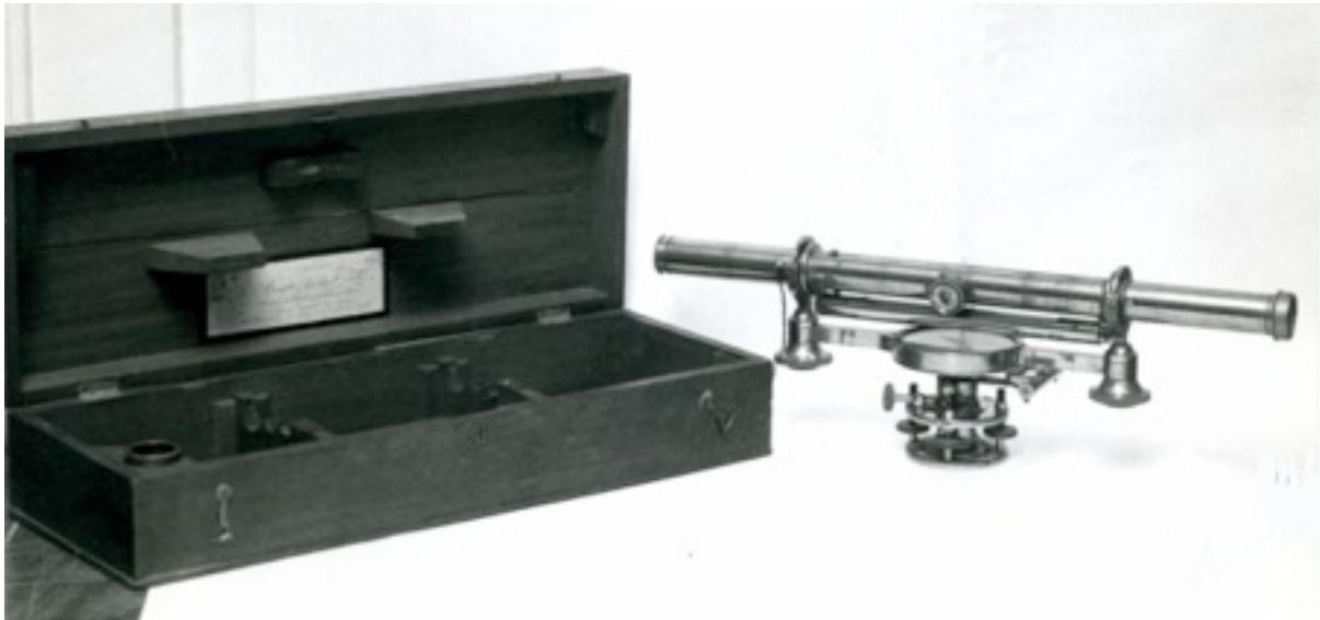
A surveyor's level with dial complete with its carrying box.
