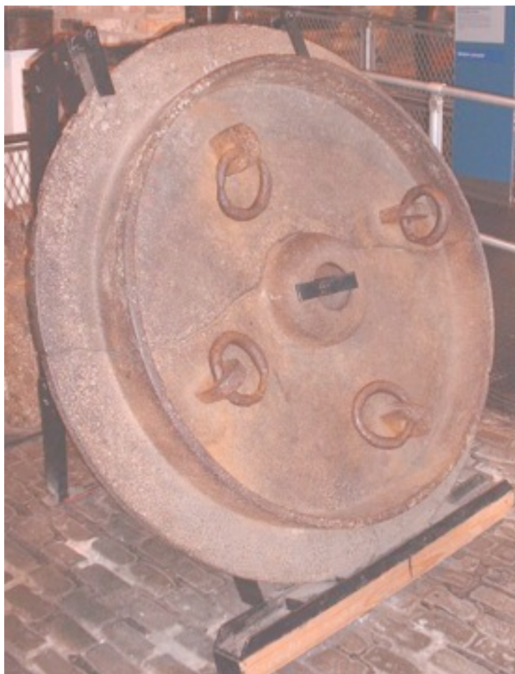
The piston from the Newcomen engine at Reel Fitz Colliery Cumbria
