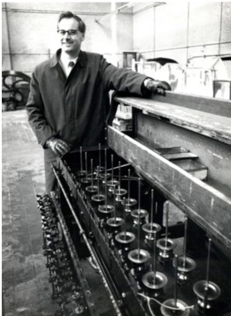
Probably an early gassing frame in which cotton yarn was passed through a gas flame to burn off any protruding fibres before the yarn was treated in the Mercerization process.
