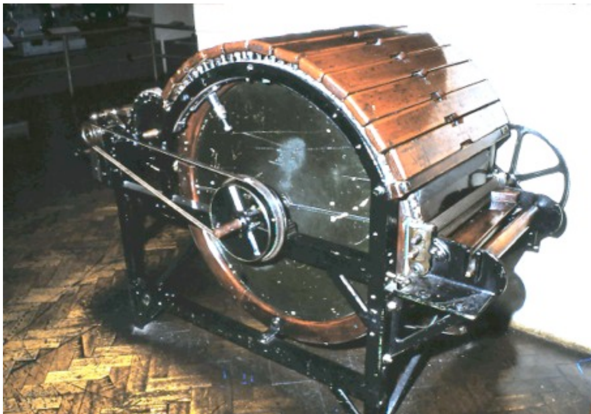
The early carding engine showing the end where the cotton was fed in.
