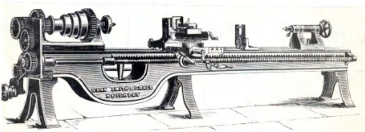
Typical large gap bed lathe.
