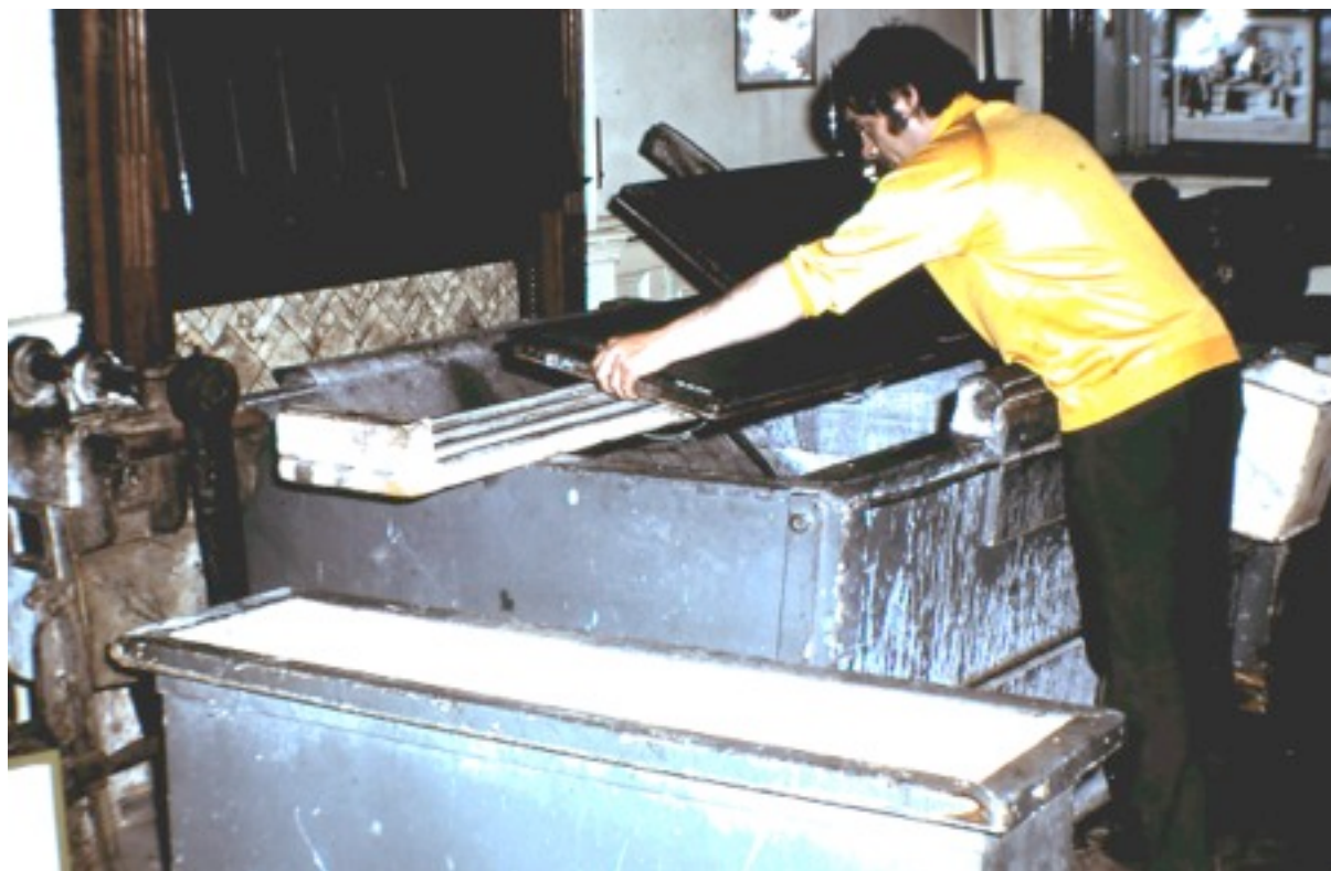
The lead-lined vat in use at Grosvenor Street for making a sheet of paper on a mould.
