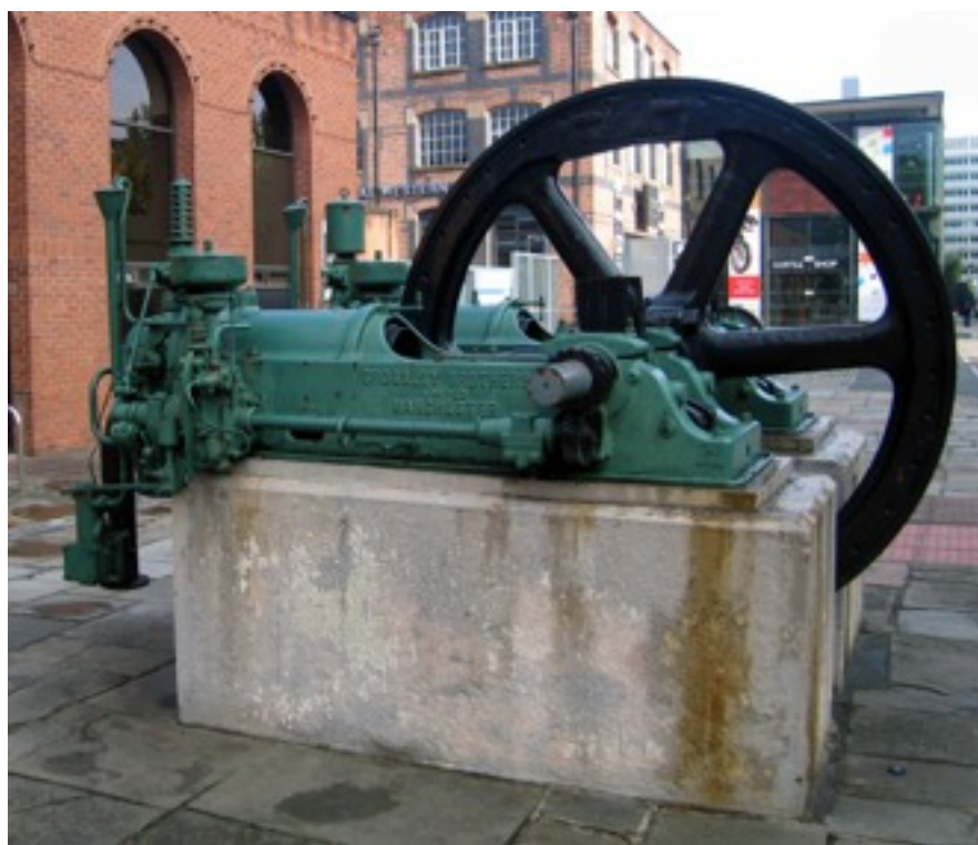
A Crossley two cylinder horizontal engine with flywheel in between the cylinders.
